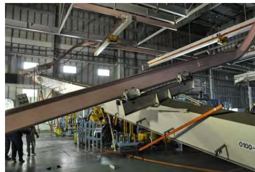
Fig. 13 Failure mode of an overhead crane (fallen rail)
