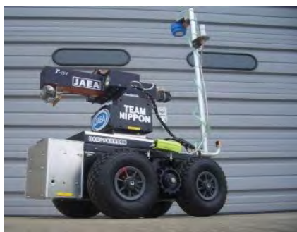
(a) Remotely controlled robot J-3 with the \gamma -eye camera
