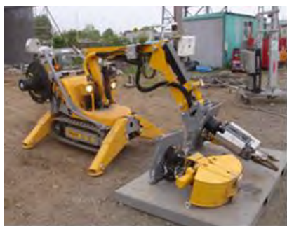
(a) BOBCAT (b) BROKK Fig.25 Remotely operated robots used to remove indoor debris
