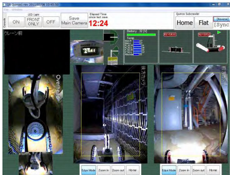
Fig.21 Operation panel of Quince
