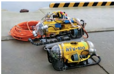
(a) Remotely operated vehicles RTV-100 and RTV-100Mk2
