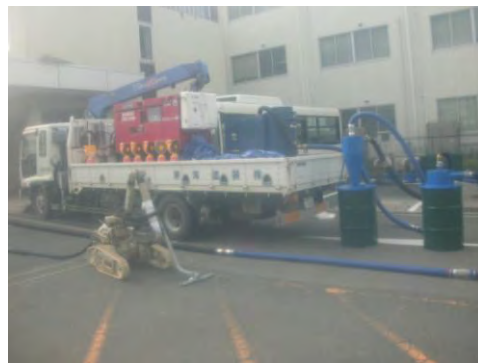
(a) 710 Warrior (a) Quince and Pelican (b) 710 Warrior equipped with a cleaner ( http://www.tepco.co.jp/en/news/110311/images/110630_4.jpg ) Fig.24 710 Warrior that was used to clean the floors in the reactor buildings
