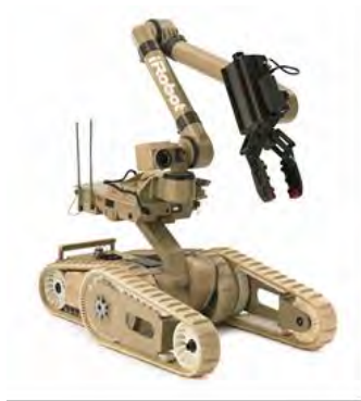
(a) 710 Warrior (a) Quince and Pelican (b) 710 Warrior equipped with a cleaner ( http://www.tepco.co.jp/en/news/110311/images/110630_4.jpg ) Fig.24 710 Warrior that was used to clean the floors in the reactor buildings
