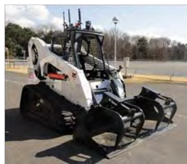
(a) BOBCAT (b) BROKK Fig.25 Remotely operated robots used to remove indoor debris
